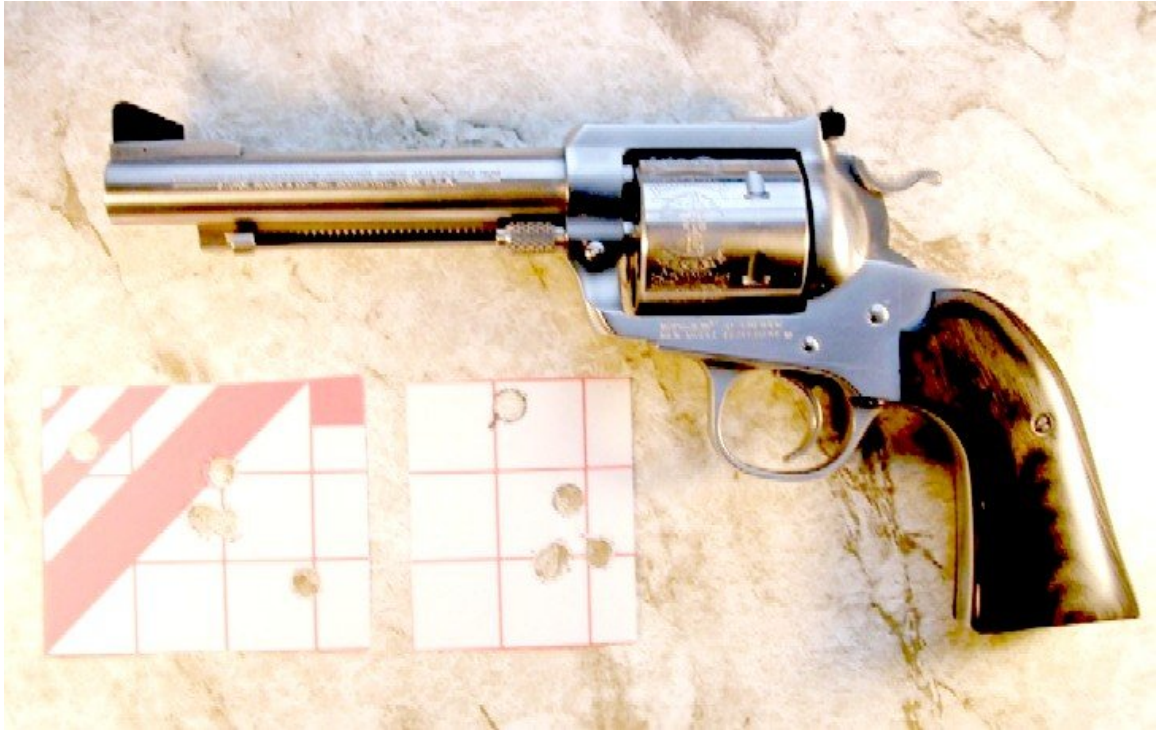
Accusport Bisley in .45 Colt. Typical 25 yard group before throating (left). Five-shot group using the same load after throating (right). On average, correct throats reduced group size by 0.6”.
